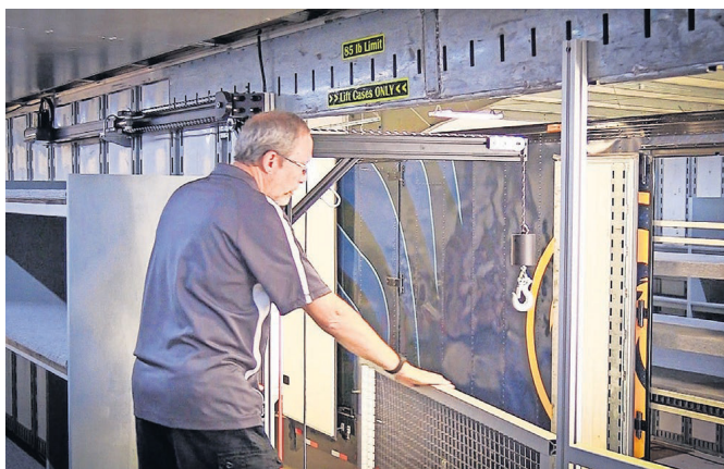
Jeff Hadley demonstrates the "tubavator," designed by Clubhouse Trailers to lift heavy instruments like tubas and sousaphones.
